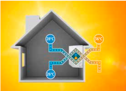
Cooling test conditions \Delta T=8^{\circ}\text{C}
