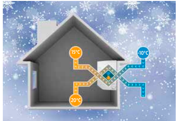
Heating test conditions \Delta T=25^{\circ}\text{C}
